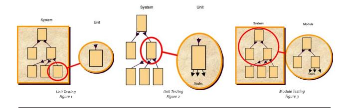
There are two primary activities in a Unit (or Module) test: Interface testing and test verification. Many projects focus the Unit Testing process on deriving inputs and expected outputs from a requirements and design base and then utilising this information to determine if the set of actual outputs matches those predicted.
